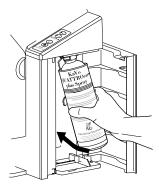
Swing the canister and adaptor back into the instrument.
