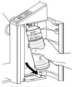
Swing the spray can and the adaptor out of the device.
