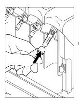
Press the handpiece, with the chuck to be serviced leading, against the tip of the chuck service coupling.
