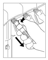
Press on the latch with a thumb and take the straight or contra-angle handpiece off by simultaneously pulling in the direction of the axis of the service coupling.
