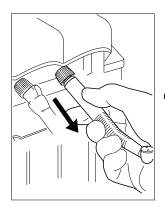
Pull the turbine in the axial direction of the service coupling, and take it off.
