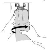
Screw the spray can into the adaptor in clockwise direction and tighten until you notice a resistance. Do not jam it.
