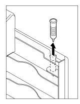
A holder for accommodating the chuck service coupling is provided in the side door. The service coupling is included in the accessories package at the time of delivery.
