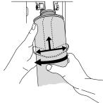
Place the spray can on the retention clip and unscrew it counterclockwise from the adaptor.
