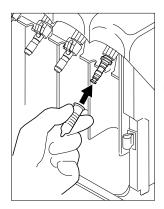
Take the chuck service coupling out and attach it to coupling service point 4 (on the far right). A MULTIflex adaptor must be mounted on the coupling.
